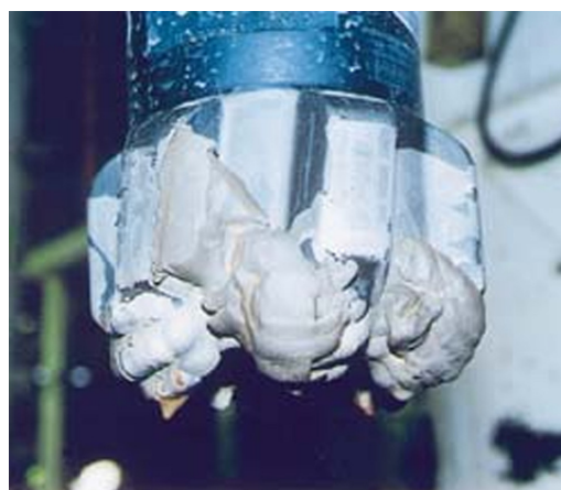
Figure 6. Drill bit showing bit balling in a laboratory test (Mensa-Wimot 1997).
