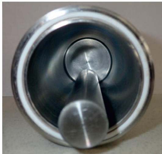
Figure 8. Accretion Test Cell – Solid Steel Bar (Błaż, 2019).
