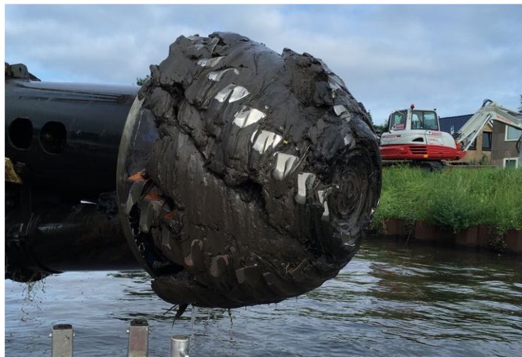
Figure 1. Blocked cutter head with highly plastic sticky clay.
