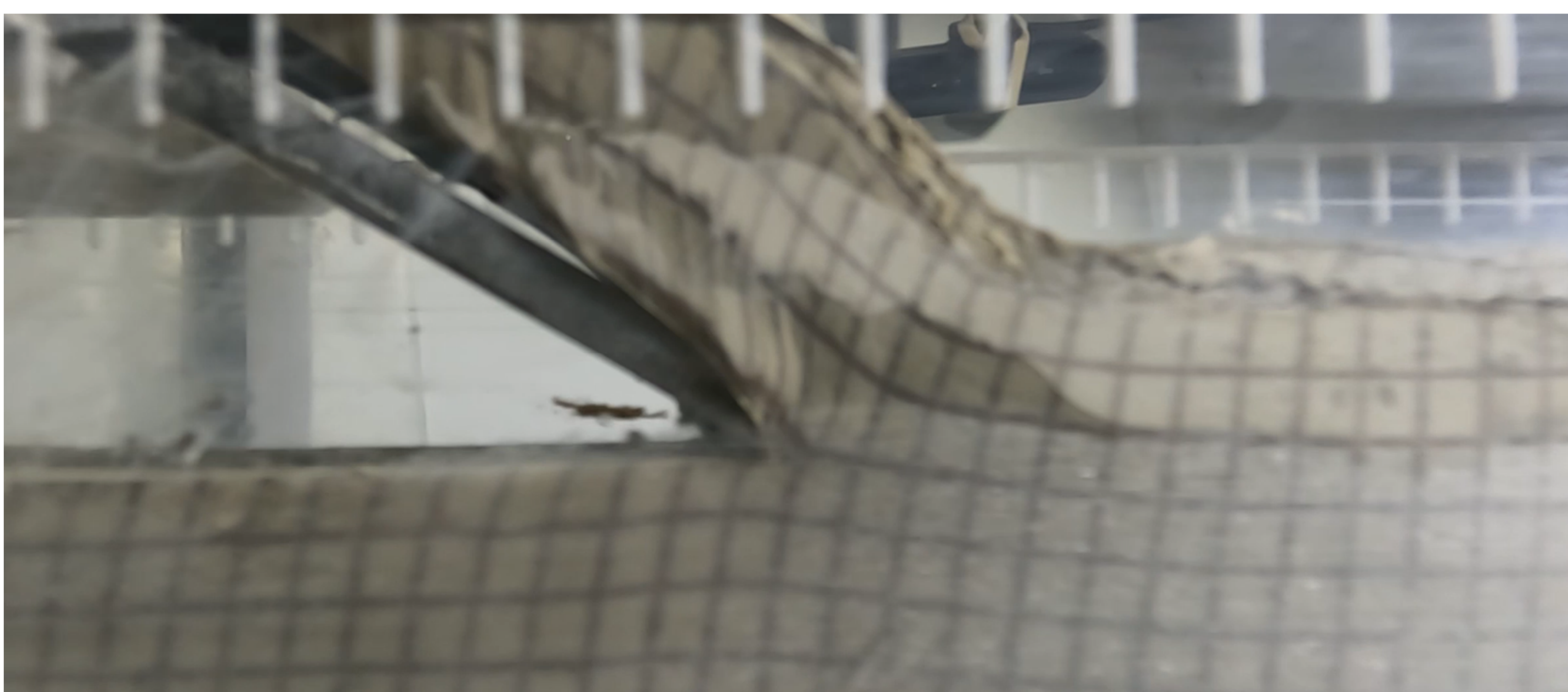
Fig. 4. Deformations visible with a grid printed on side of the clay sample.
