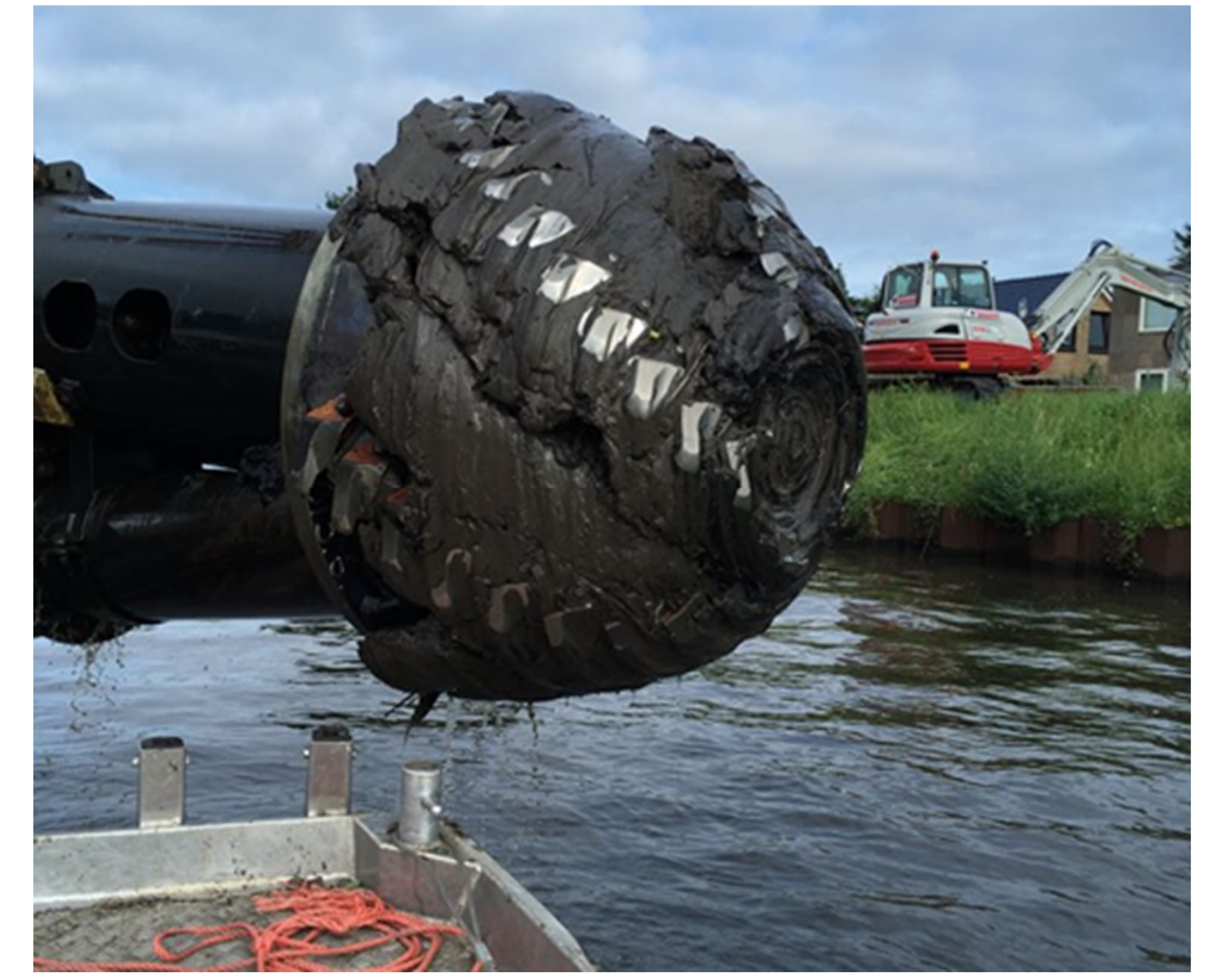
Fig. 1. Example of a clogged cutter head.
