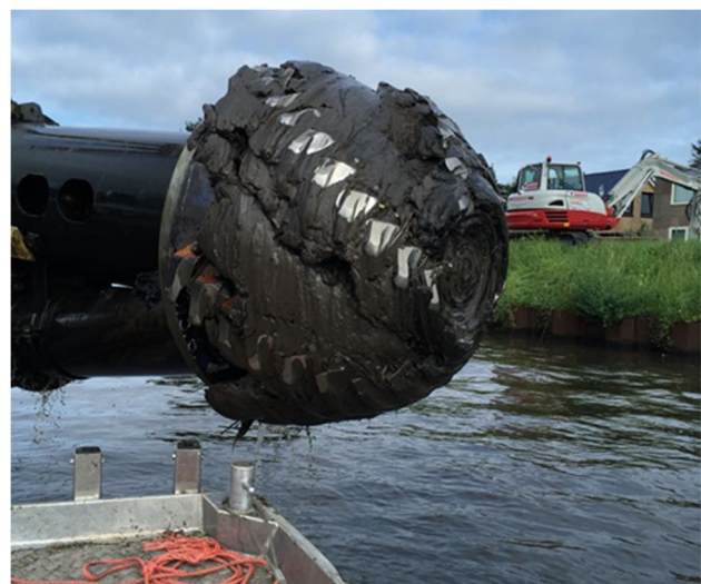
Figure 1 Clogged cutter head in highly plastic clay
